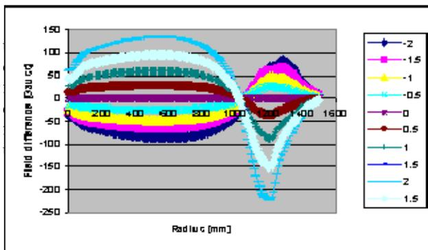
Figure 6: Coil B3 response as a function of radius for different current densities showing non linearities
