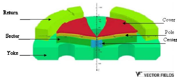
Figure 1: Main parts of C70
