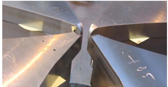
Figure 11: The cover tips at center are very accurately machined to tailor the central field for injection.
