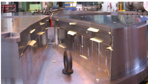
Figure 9: Intermediate assembly is performed at various stages of machining to ensure final assembly tolerances.
