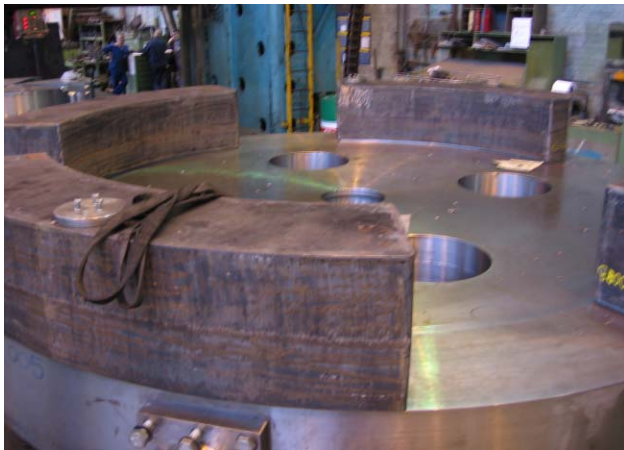
Figure 8: Cast returns are installed on the yoke to machine all cylindrical surfaces on a 5m lathe
