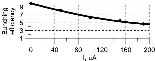
Figure 6: Bunching efficiency versus beam current
