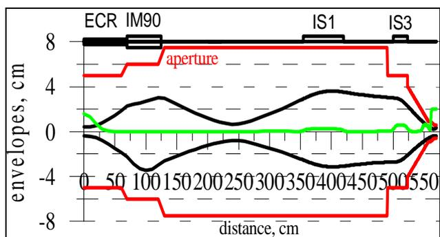
Figure 3: <sup>48</sup>Ca<sup>6+</sup> beam envelopes along the beam line. Beam current 190 μA
