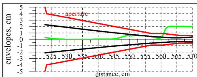
Figure 4: <sup>48</sup>Ca<sup>6+</sup> beam envelopes near inflector
