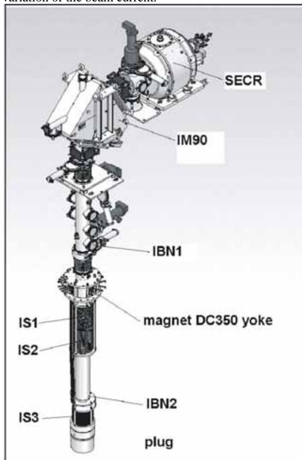
Figure 1: Beam line layout
