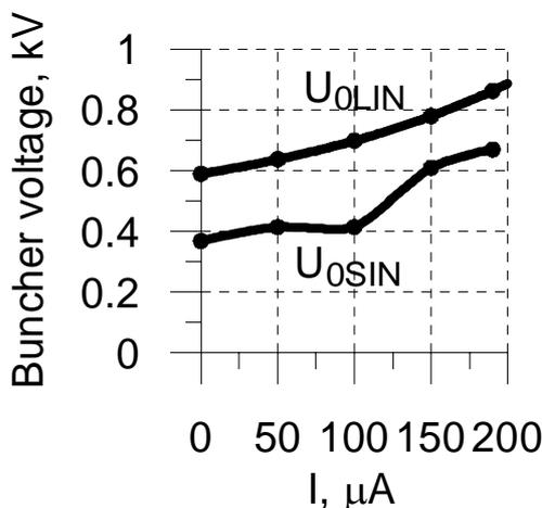
Figure 7: Bunchers voltage for various beam currents
