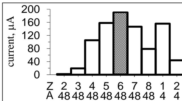
Figure 2: <sup>48</sup>Ca beam charge state distribution
