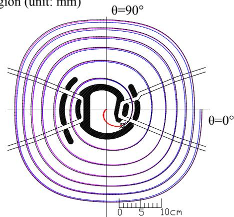
Figure 2: Central rays of three particles with different initial phases in central region, the phase width is 40°; with the central ray through the inflector together
