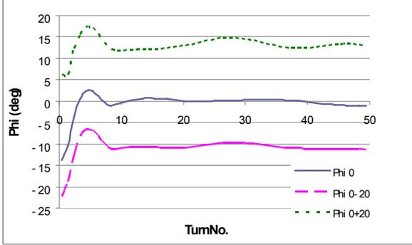
Figure 3: Phase history as a function of turn number at the position of  $\theta=90^\circ$  (see Fig. 2) for three particles with different initial phase
