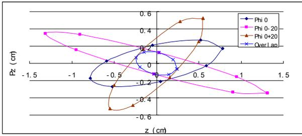
Figure 5: The vertical acceptance results, the “overlap” is the acceptance at the matching point for the CYCIAE-100 cyclotron with the 40° RF phase width
