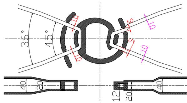
Figure 1: Two sections schematic (up- horizontal; down- vertical) of the electrode structure for the CYCIAE-100 central region (unit: mm)
