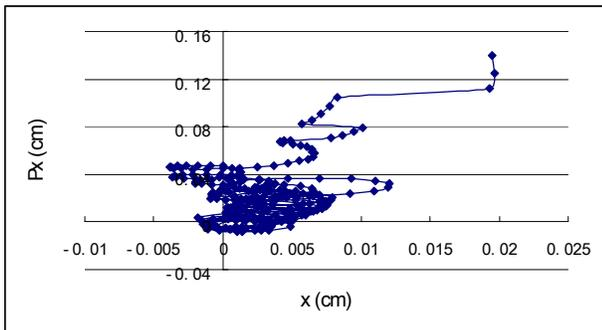
Figure 4: Radial phase space of AEO plotted at the position of the center line of the first dee ( $\theta=0^\circ$ ), where  $x=r-r_{seo}$ ,  $P_x=P_r-P_{rseo}$
