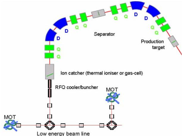
Figure 1: Schematic layout of the KVI RIB facility
