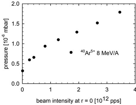
Figure 4: Pressure as a function of the injected beam intensity for  $^{40}\text{Ar}^{5+}$  accelerated to 8 MeV per nucleon.
