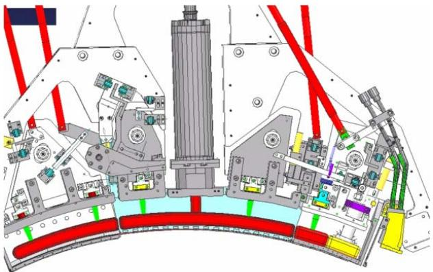
Figure 2: Top view of the new ESD design. The beam enters from the right. The red curved parts represent the cathode.
