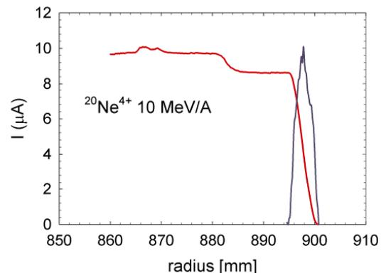
Figure 3: Beam intensity as a function of radius and radial profile of the extracted beam measured with the radial probe at the exit of the ESD.
