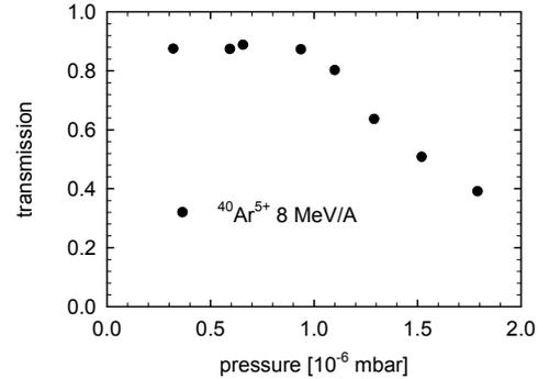
Figure 5: Transmission as a function of pressure for  $^{40}\text{Ar}^{5+}$  accelerated to 8 MeV per nucleon.
