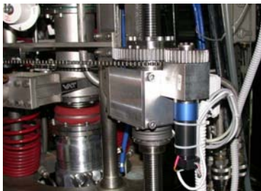
Figure 5: the new mechanic and the DC motor.
