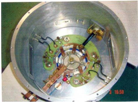
Figure 6: Input circuit (assembled) for amplifier
