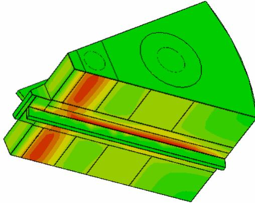
Figure 2: The power loss distribution on the RF cavity
