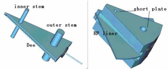
Figure 1: The RF cavity model of CYCIAE-100 with two stems
