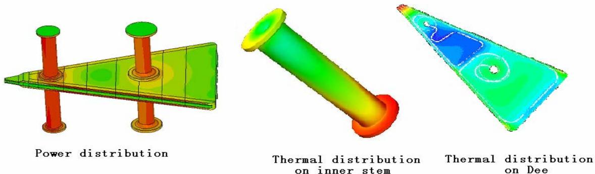
Figure 3: Thermal distribution of inner stem and Dee
