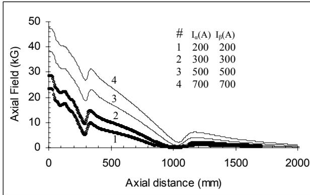
Figure 5. Axial field distribution [— calculated, oo measured]
