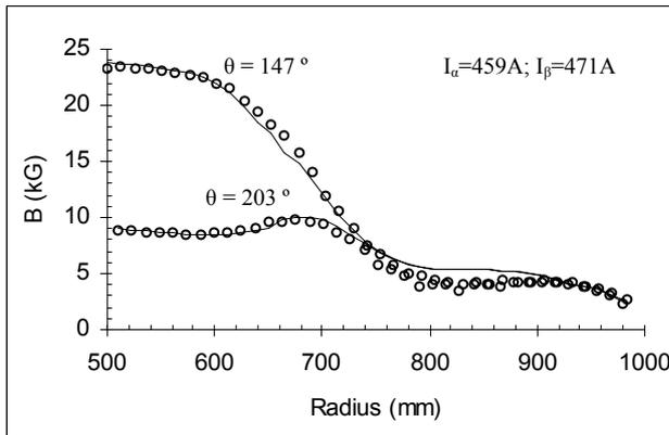
Figure 6. Comparison of Edge iron field at two different angles [— calculated, oo measured]
