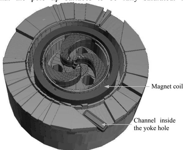
Figure 1. Lower half portion of the magnet.
