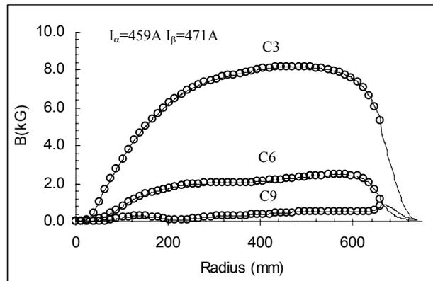
Figure 4. Measured and calculated amplitude of the 3<sup>rd</sup>, 6<sup>th</sup> and 9<sup>th</sup> harmonics, as function of the radius at the listed coil currents [— calculated, oo measured].
