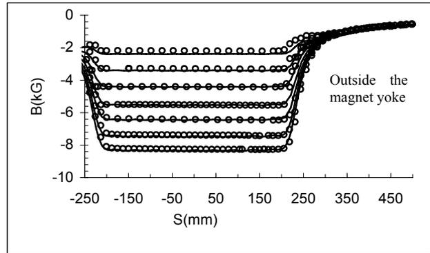
Figure 7. Field inside the active channel. [— calculated, oo measured]
