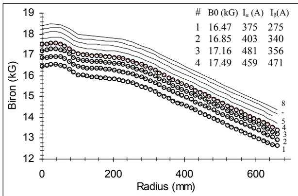
Figure 2. Average Iron field profile for the listed coil currents. Top 4 curves are obtained from simulation. [— calculated, oo measured]
