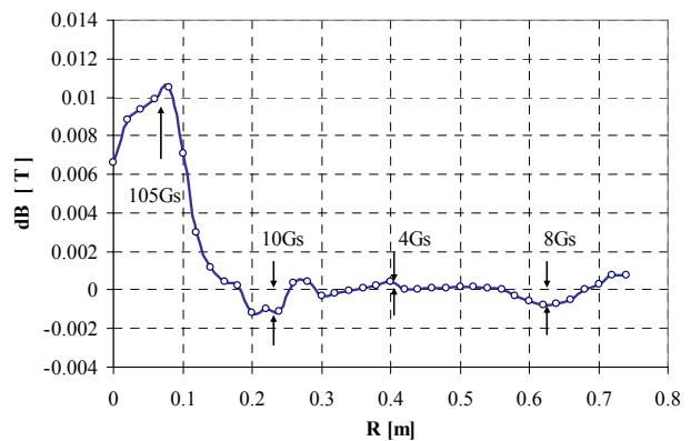
Figure 3: The deviation of the measured average magnetic field from the calculation results,  $1.43\text{T}$
