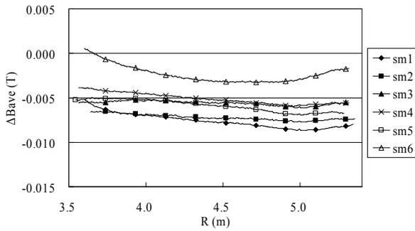
Figure 4: The average magnetic field of each sector magnet at a main coil current of 5000 A.
