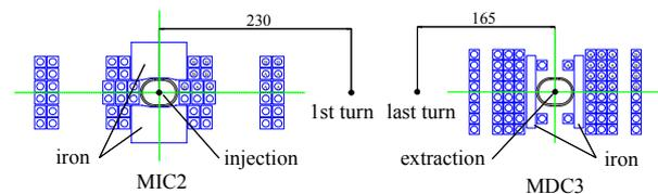
Figure 2: Cross-sections of the MIC2 and the MDC3.
