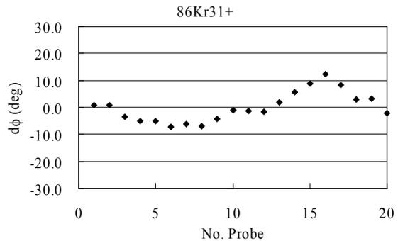
Figure 7: Measured phase excursion of the  $^{86}Kr^{31+}$  beams accelerated in the magnetic field of the calculated trim coil currents.
