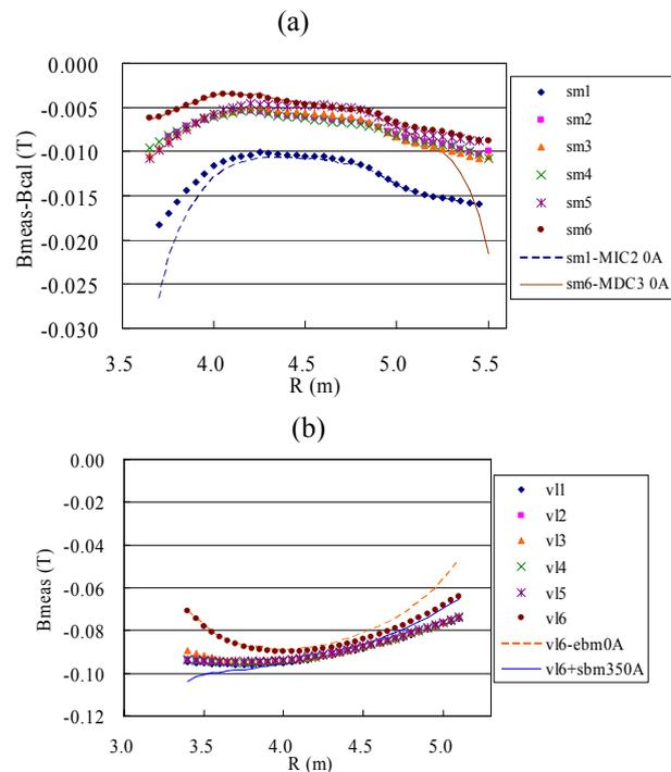
Figure 3: Magnetic field distributions along (a) the sector center lines and (b) the valley center lines.
