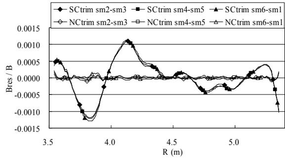
Figure 6: Relative residuals in the fitting of the isochronous magnetic field for the 345 MeV/u  $U^{86+}$  beam.
