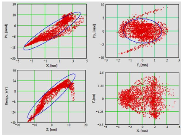
Figure 3: Effective emittance of the beam at the BDS entrance, 260  $\mu\text{A}$  beam intensity.
