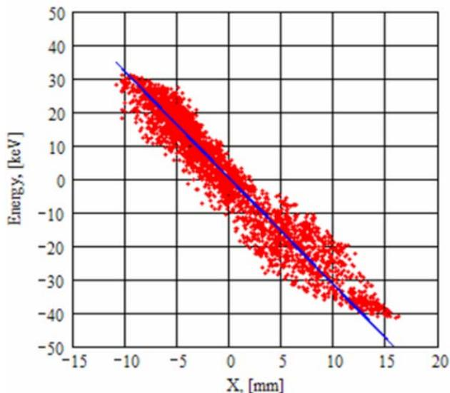
Figure 6: Dispersion estimation at injection point, 130  $\mu\text{A}$  beam intensity.
