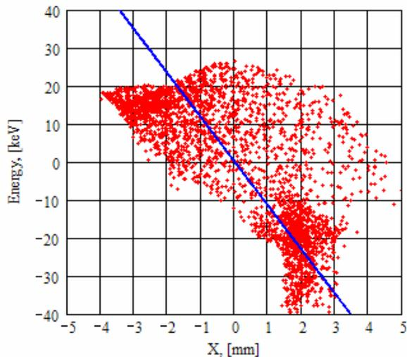
Figure 4: Dispersion estimation, 260  $\mu\text{A}$  beam intensity.
