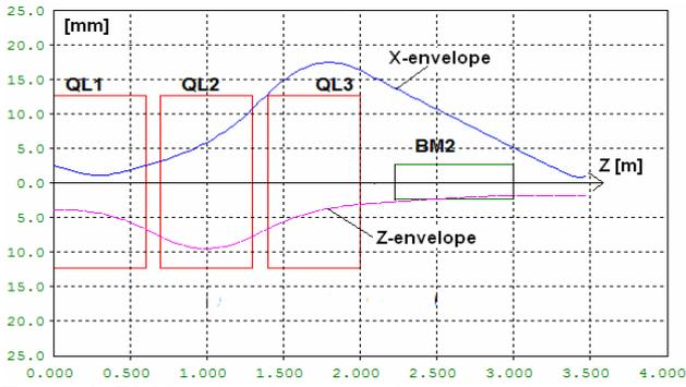
Figure 6: RMS carbon beam envelopes outside the cyclotron. Z is a length of the beam way from the entrance into the first lens QL1.
