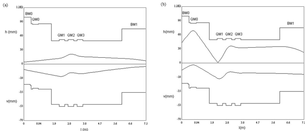
Figure 3: The horizontal (h) and vertical (v) envelopes of (a) the 65 MeV  $H^+$  test ion beam, and (b) the 32 MeV  $H^+$  test beam along the front extraction system. They are given from the entrance plane of the bending magnet (BM0) to the exit plane of the main bending magnet (BM1).
