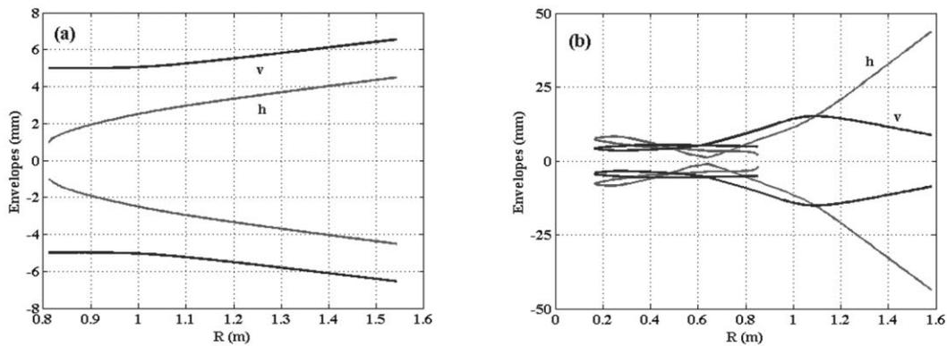
Figure 2: The horizontal (h) and vertical (v) envelopes of (a) the 65 MeV  $H^+$  test ion beam, and (b) the 32 MeV  $H^+$  test beam as functions of the distance from the center of the machine. They are given from the stripping foil (F1) to the entrance plane of the bending magnet (BM0).
