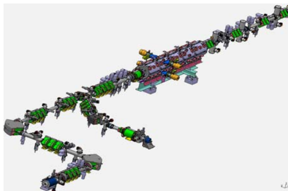
Figure 1: View of injector-1 (LEPT, RFQ and MEPT)
