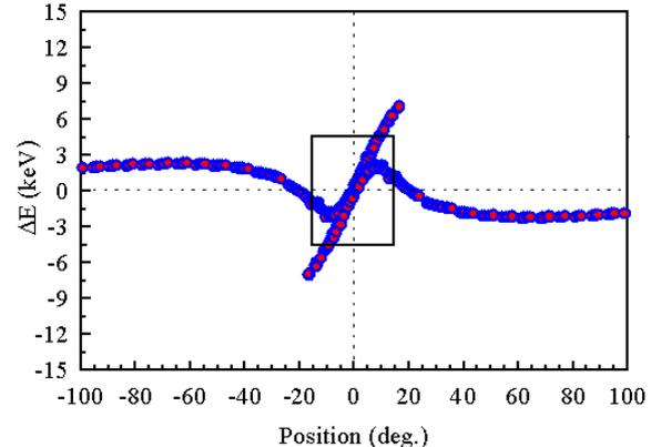
Figure 6: Phase space plot at the beam waist.
