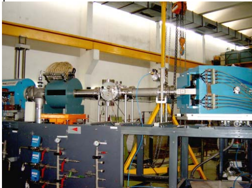
Figure 5: ECRIS 1 along with analysing magnet (AM2), installed on the high bay of cyclotron building.
