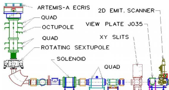
Figure 1: Injection beam line layout. The distance from ARTEMIS-A to the analysis magnet is about 2.2 m. The line continues horizontally, then bends upward for injection into the K500.
