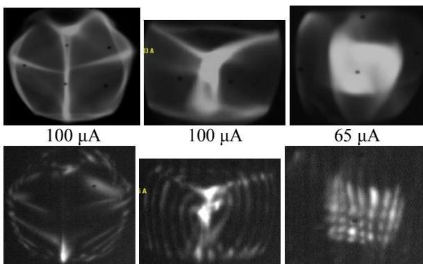
Figure 2: Images of <sup>40</sup>Ar<sup>7+</sup> beam from Artemis-B using electrostatic lenses. At top are images of undisturbed beam. At bottom, a blocking grid of 1.5 mm holes located 4 mm apart, is inserted 79 cm upstream of the image. The source tune remains the same; all differences between the image pairs results from changing the settings of the electrostatic doublets before the analysis magnet.
