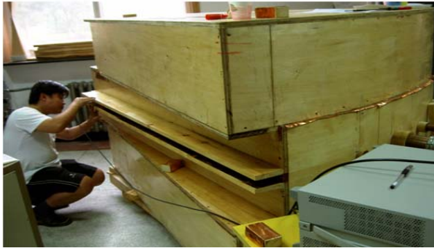
Figure 12: Cold test of the RF wooden model cavity
