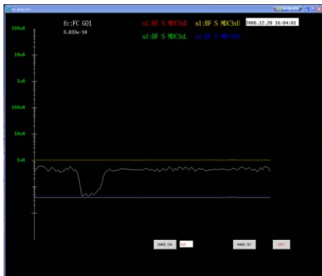
Figure 4: Monitor view of beam current (faraday cup and baffle slits).
