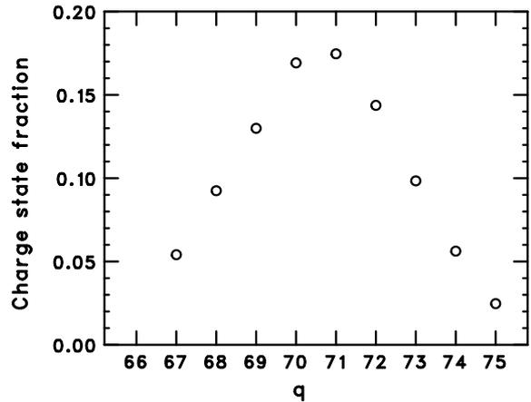
Figure 4: Charge state distribution of uranium at 11 MeV/nucleon stripped by 0.3- $\text{mg}/\text{cm}^2$ -thick carbon foil. The horizontal and vertical axes indicate the charge state and charge state fraction of uranium ions, respectively.
