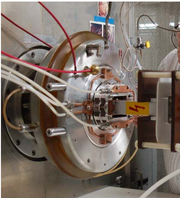
Figure 3: Installation of the source at the test stand showing also the ridged wave guide and the HV break.
