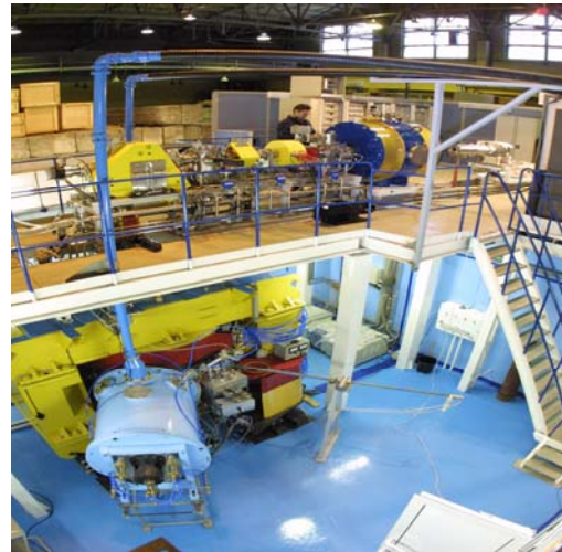
Figure 1. IC100 cyclotron. Shown are the SC ECR source, injection line, magnet and resonance cavity.
