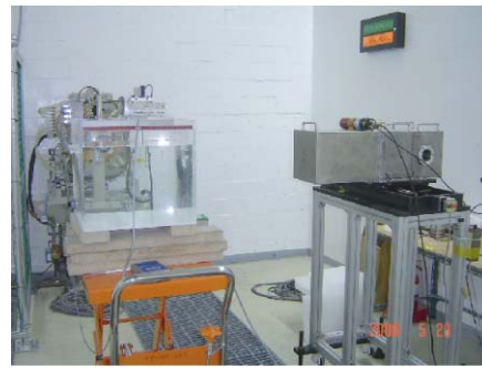
Figure 7: A setup to measure the prompt gamma distributions. Water phantom and the collimator system are shown. The CsI detector is taken out to count background radiation.
