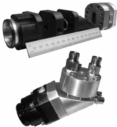
Figure 1. Cyclotope targets. Top, disassembled prototype. Bottom, final target in irradiation position.
