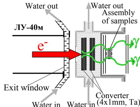
Figure 4: Activation circuit scheme of experimental Zn targets.
