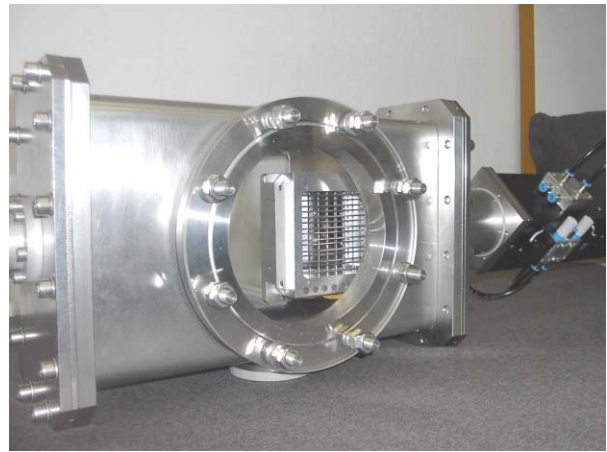
Figure 9. Extraction chamber with profilometer
