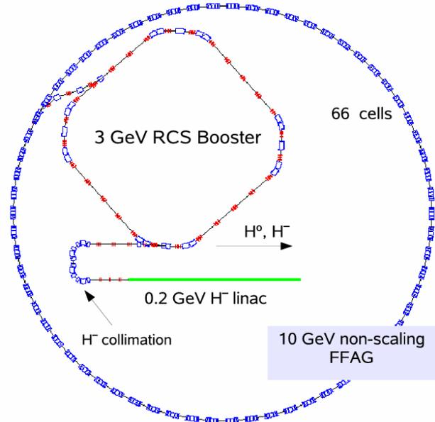
Figure 1: Layout drawing of the 4 MW, NFFAG driver.
