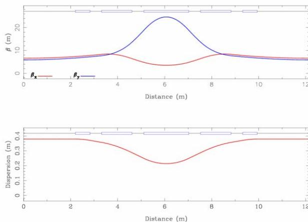
Figure 3: Small amplitude, betatron and dispersion functions for the NFFAG, 10 GeV orbit.
