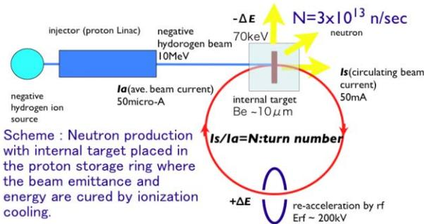
Figure 4: Schematic layout of ERIT.
