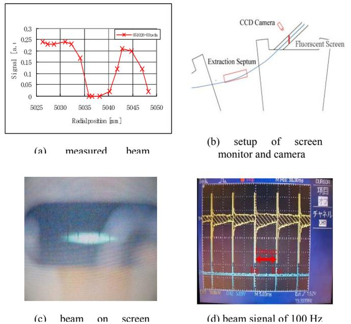
Figure 3: Results of the beam extraction crosses resonance at a beam energy slightly above that at injection.
