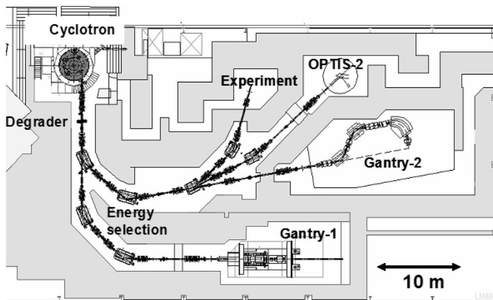
Figure 1. The proton therapy facility at PSI, with the SC cyclotron and beam lines to three treatment areas and one area for experiments.
