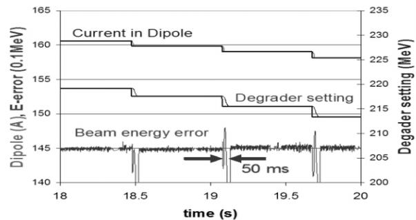
Figure 6. A fast sequence of beam energies is shown. The energy set by the degrader is given on the right axis and on the left axis the magnet current in the analyzing magnet and the beam position at the dispersive focus are shown. The latter has been expressed as the energy mismatch in units of 0.1 MeV (displayed with an offset of 145 MeV). During an energy change the beam is switched off, causing the wiggles in this signal.
