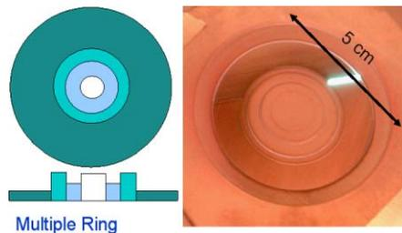
Figure 8: A foil consisting of multiple rings is used as second scattering foil (courtesy Marc-Jan van Goethem). The foil is made by laser ablation at the Fachhochschule Aargau (CH).
