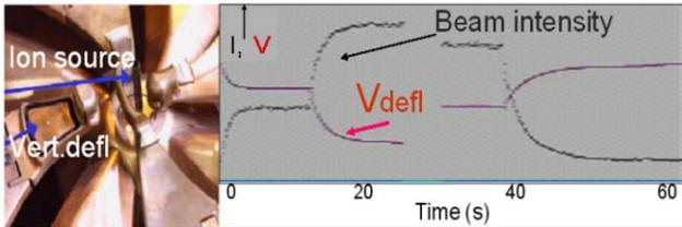
Figure 3. The vertical deflector used for intensity control and beam on/off switching.
