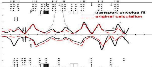
Figure 4. Calculated [3] and measured beam envelopes and dispersion (dotted) of the undegraded 250 MeV beam. Above the horizontal axis the vertical beam size is shown, below indicates the horizontal beam size. The “T” symbols indicate the measured beam widths.
