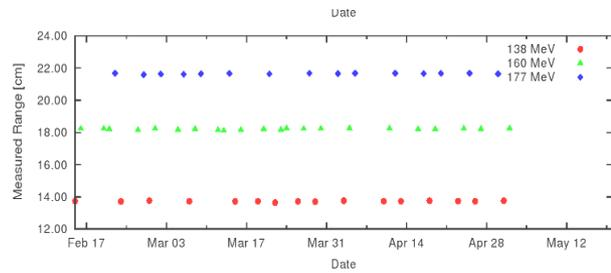
Figure 5. Results of the daily QA checks of ranges of 138 MeV, 160 MeV and 177 MeV protons at Gantry-1. The measured ranges are constant within a standard deviation of 0.3 mm, 0.4 mm and 0.4 mm (courtesy Jürgen Salk).
