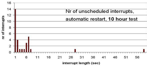
Figure 2. Unscheduled interrupts during a test of 10 hours running time.
