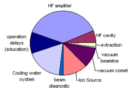
Figure 10. The subsystems causing unscheduled down time during the patient treatment period Feb.-May 2007.
