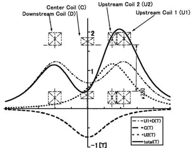
Figure 4: Simulated magnetic field distribution.
