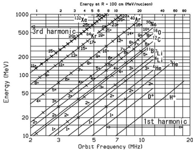
Figure 2: The resonance conditions for acceleration of the RCNP AVF cyclotron.
