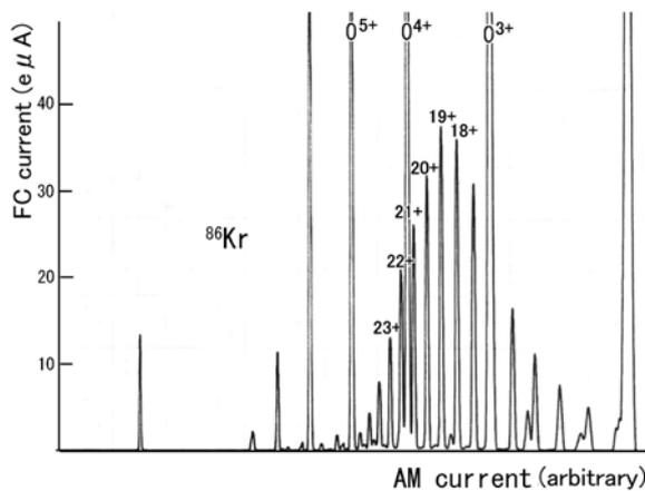
Figure 5: Charge state distribution of  $^{86}\text{Kr}$  ions with 700W RF and oxygen mixing.
