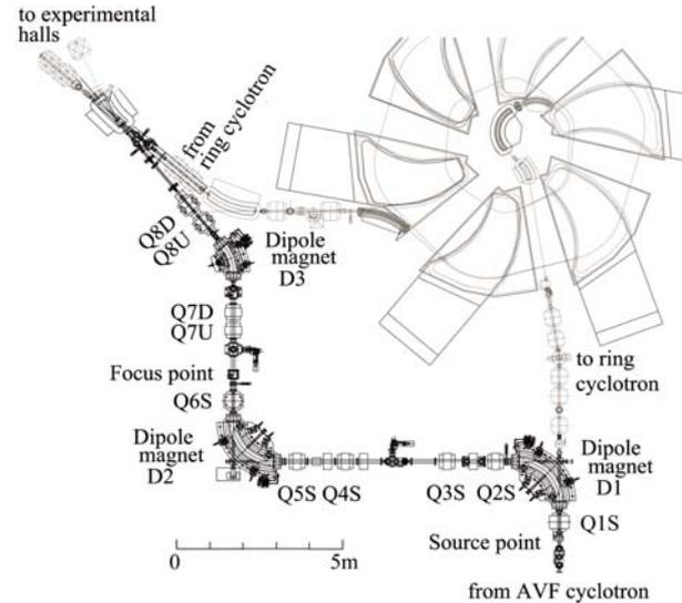
Figure 7: Schematic layout of the beam line to analyze the quality of the beam from the AVF cyclotron as well as to directly deliver low energy and high intensity beams to experimental halls of the ring cyclotron.
