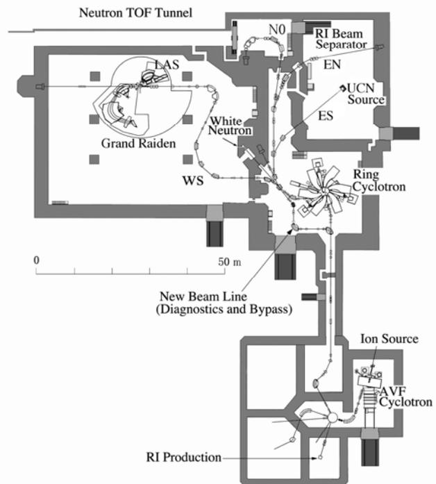
Figure 1: Layout of the RCNP cyclotron facility.
