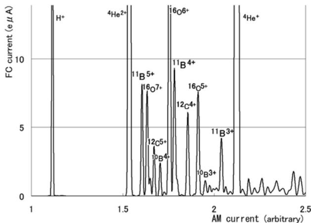
Figure 6: Charge state distribution of  $^{11}\text{B}$  ion.
