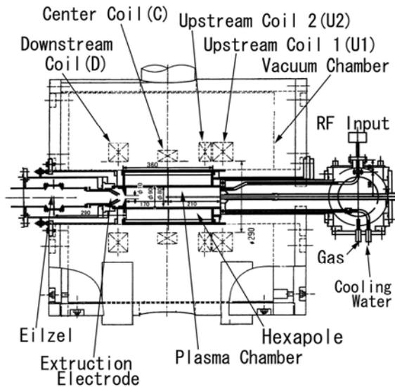
Figure 3: Cross sectional view of liquid-helium free 18 GHz superconducting ECR ion source.
