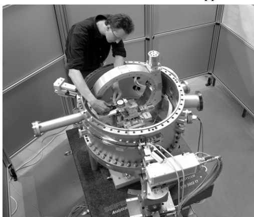
Figure 4: View on the on-line 4-circle X-ray diffractometer, commissioned at the end of 2005.
