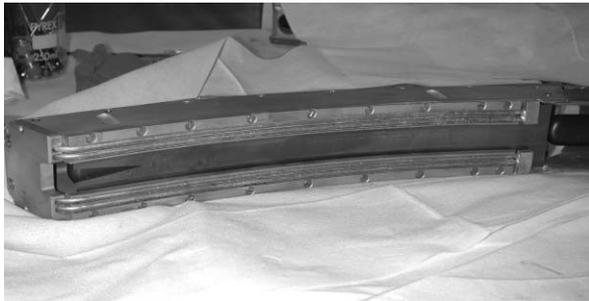
Figure 10: New deflector provided with direct cooling of the septum
