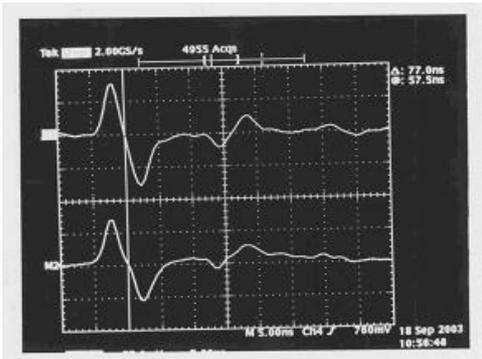
Fig.4. Typical two signals from Probe No.1(upper) and No.2 (lower) for 40 MeV  $\alpha$ -beam at intensity of 0.5  $\mu\text{A}$ .
