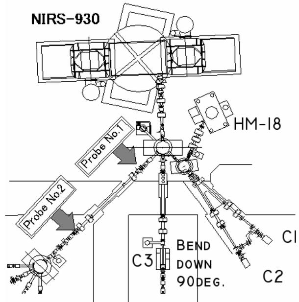
Fig.2. Schematic drawing for beam pick-up probe arrangement in transport line.
