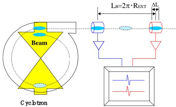
Fig.1. Layout of beam bunch distribution on transport line for acceleration mode of  $h = 1$  and  $h = 2$ .
