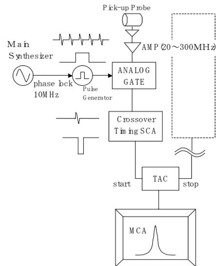
Fig.3. Block diagram of signal processing electronics for MCA. A set of two signals from amplifiers are thin out by analog-gate module, see in text.
