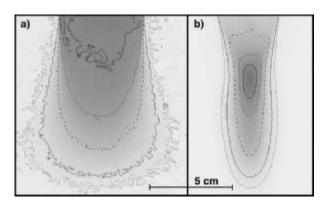
Figure 3: Isodose profiles for a 5 cm diameter 20 MV electron beam in a polystyrene phantom without (left) and with (right) an applied 3T field along the incident beam direction (vertical axis).
