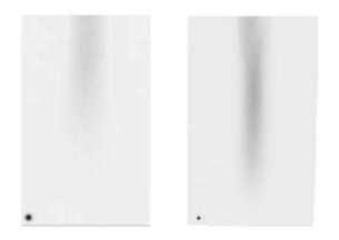
Figure 2: Film-density scans of a 5 cm diameter collimated 50 MeV electron beam in a polystyrene phantom without (left) and with (right) a 3T applied field.
