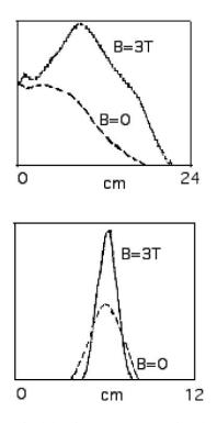
Figure 4: Optical density scans, proportional to dose, taken along the beam axis (top) and perpendicular to the beam axis (bottom) near the maximum in the magnetically-confined 50 MeV electron beam profile (Fig. 2)
