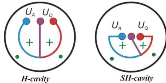
Figure 2: Two  $H$ -cavity options for the RFQ-DTLs.
