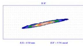
Figure 7: Phase portrait, at exit from the first section, in X-X' plane.
