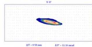
Figure 8: Phase portrait, at exit from the first section, in Y-Y' plane.
