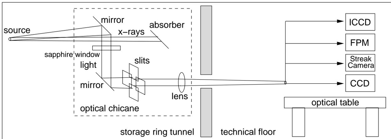
Figure 2: Schematic layout of the Optical Diagnostic Beamline viewed from side on.
