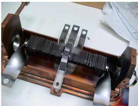
Figure 4: An ISAC target unit capable of handling up to 17 kW of stopped primary beam power.
