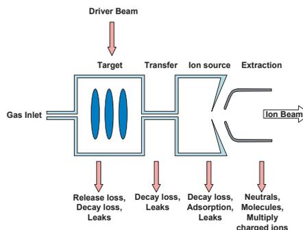
Figure 2: A schematic representation of the ISOL method and the major associated loss channels.
