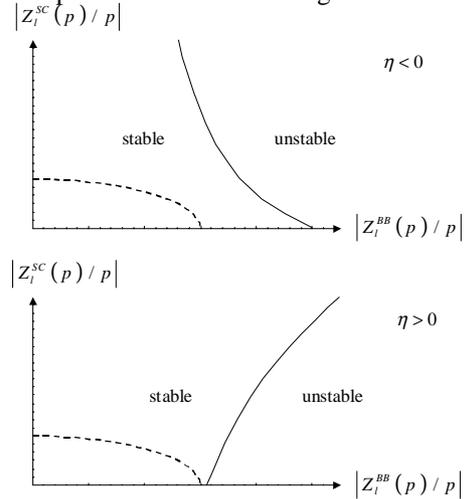
Figure 3: Stability diagram for the LMC instability
