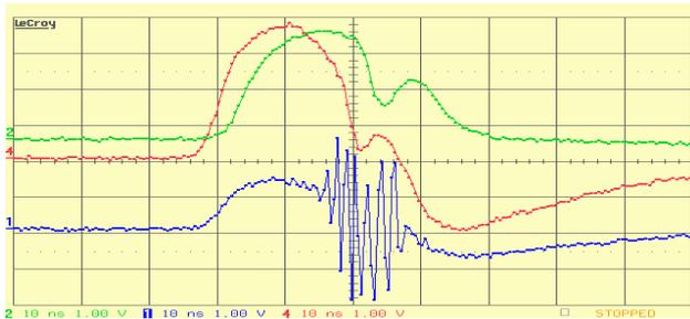
Figure 1: Single-turn signals from a wide-band pick-up. From top to bottom:  $\Sigma$ ,  $\Delta x$ , and  $\Delta y$ . Time scale: 10 ns/div.
