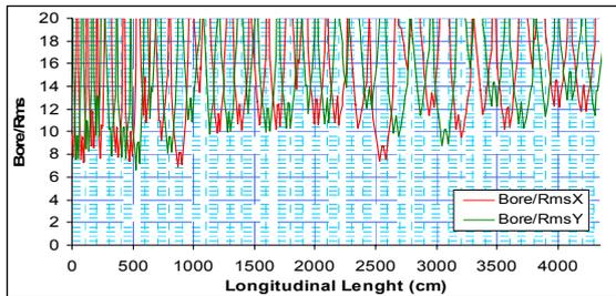
Figure 4 Cavity and quadrupole bore to rms beam size ratio.
