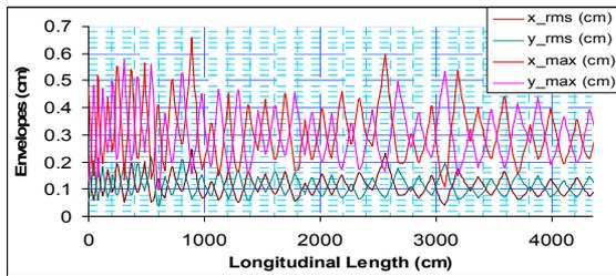
Figure 3 Beam amplitude rms and max along the linac.
