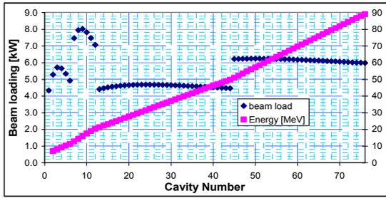
Figure 2 Beam loading per cavity and synchronous energy as function of cavity
