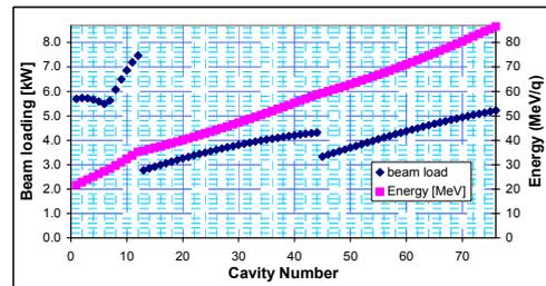
Figure 6 Beam Loading and synchronous Energy in the case of  $a/A=1/3$ .
