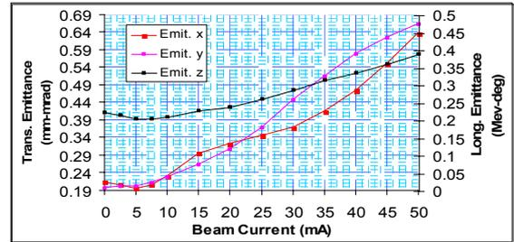
Figure 5 Output Emittance vs. beam current.
