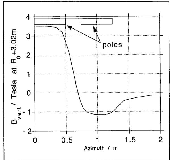
Figure 1. FFAG—Midplane Field at Extraction
