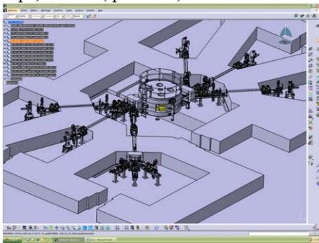
Figure 3: Beam transport lines
