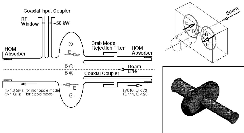
Figure 2: Concept of the squashed-cell crab cavity.
