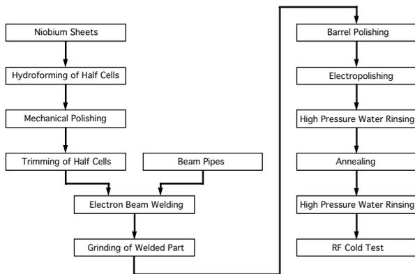
Figure 3: Fabrication and surface preparation procedure.
