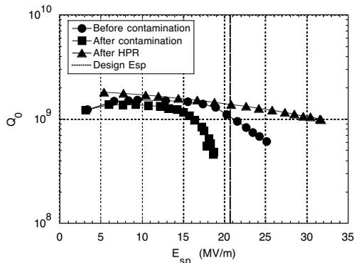
Figure 5: Effect of high pressure ultrapure water rinsing.
