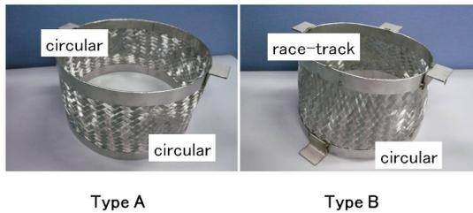
Figure 3: Two types of RF shields for investigation of their movability.
