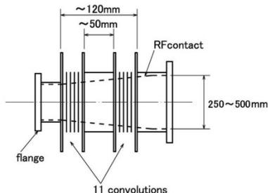
Figure 1: Basic structure of the bellows joints.
