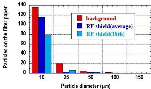
Figure 6: Dust generation from the RF shield.
