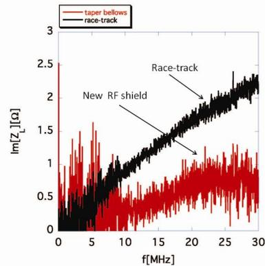
Figure 7: Imaginary parts of the longitudinal impedances for the race-track aperture and for the new RF shield, respectively.
