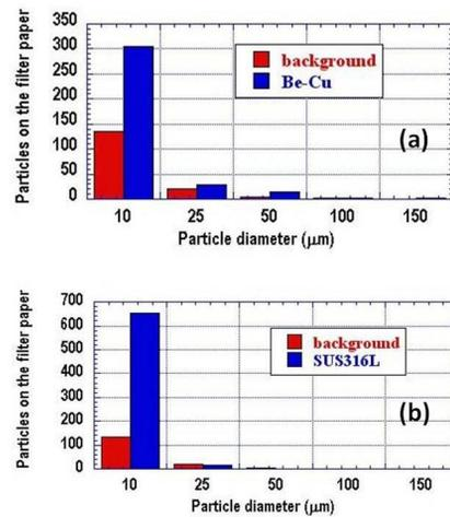
Figure 5: Dust generation due to abrasion; (a) for Be-Cu, (b) for SUS316L.
