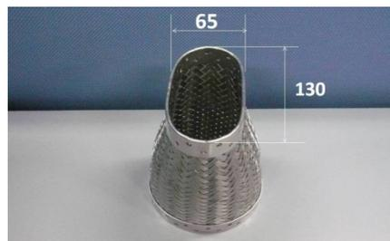
Figure 2: Example of the newly developed RF shield.
