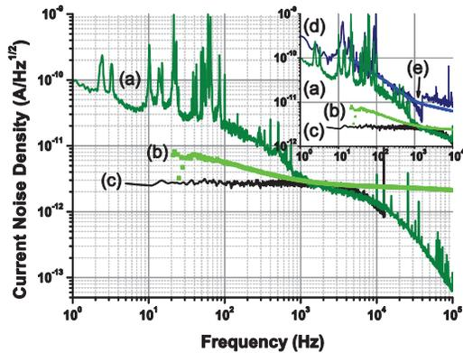
Figure 3: Measured (a) and calculated (b) current noise of the welded pick-up coil with Nanoperm M-764-01 core as well as the measured current noise of the SQUID sensor with rf-shunted input (c). The inset compares the measured (a) and calculated (b) current noise of the welded coil with Nanoperm M-764-01 core with the measured (d) and calculated (e) current noise of the DESY-CCC pick-up coil with Vitrovac 6025 F core.
