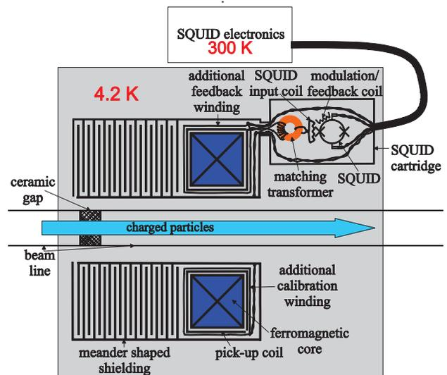
Figure 1: Circuit diagram of the CCC.
