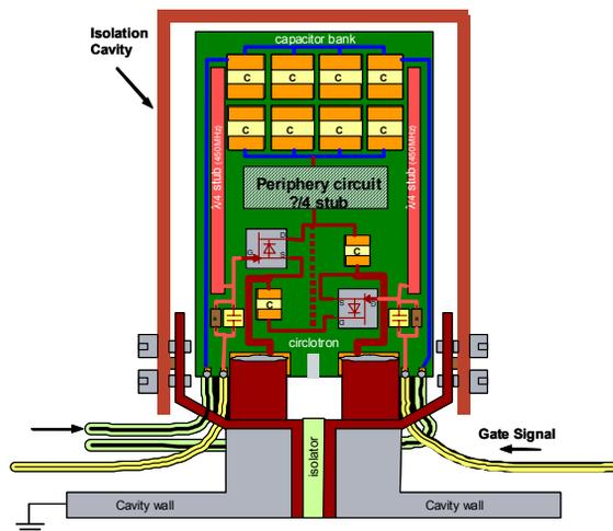
Figure 6: RF module including shield box
