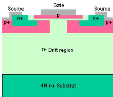
Figure 4a: SiC vJFET cell structure
