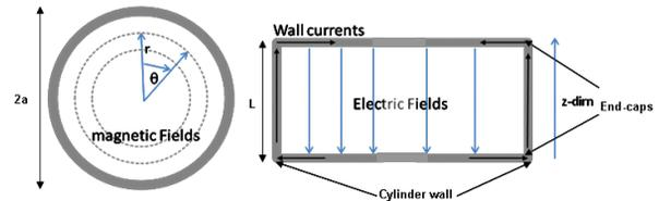
Figure 2: RF fields and currents in a pillbox cavity.
