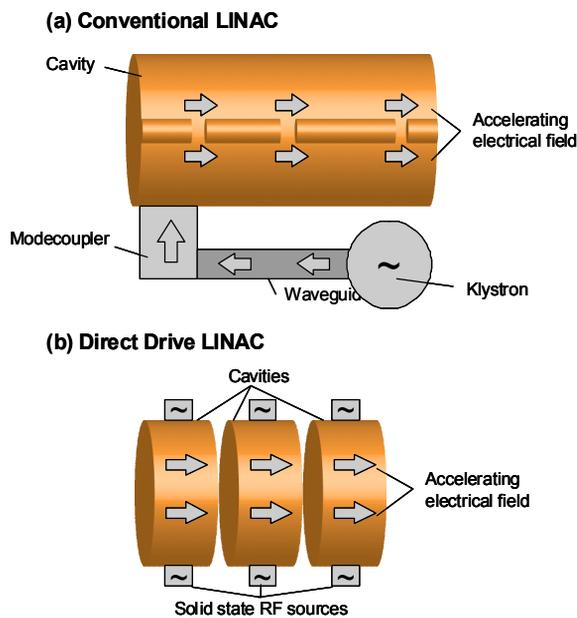
Figure 1: Conventional and direct RF cavity drive.
