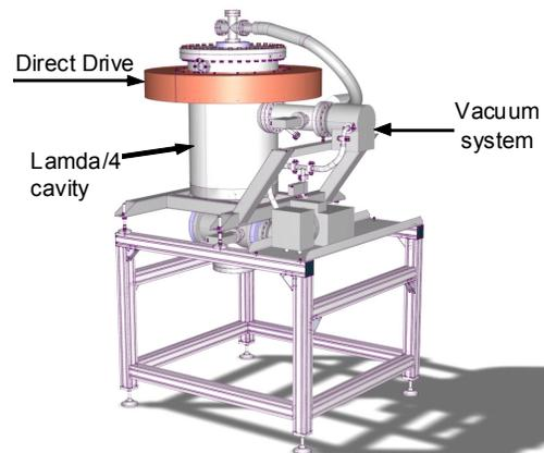
Figure 6. The direct drive experimental cavity.
