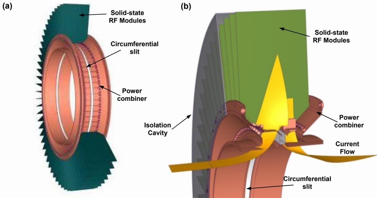
Figure 3a-b: Arrangement of RF modules across a current injection slit.
