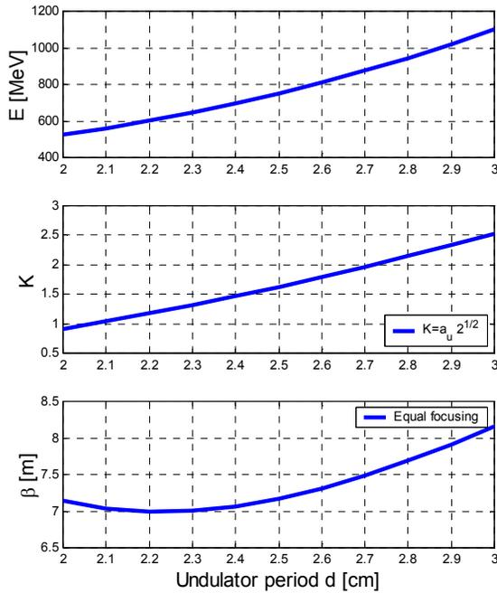
Figure 2: Electron energy  $E$ , undulator parameter  $K$  and equal-focusing  $\beta$ -function as functions of the undulator period  $d$ .  $H_c=13\text{kOe}$ , the undulator gap  $g=1\text{ cm}$ .
