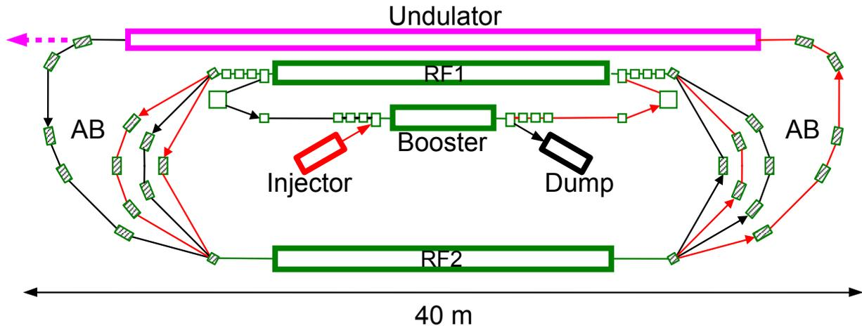
Figure 1: The scheme of ERL with FEL. RF1 and RF2 – RF accelerating structures, AB – achromatic bends. Red arrows – accelerating “fresh” beam, black arrows – decelerating used beam.
