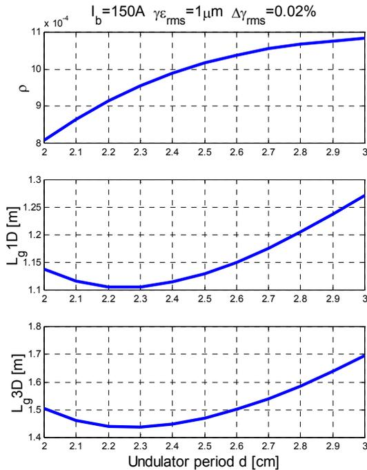
Figure 3: The Pierce parameter  $\rho$ , one-dimensional gain length  $L_{g1D}$  and actual gain length  $L_{g3D}$  as functions of the undulator period  $d$ .  $L_{g3D}$  was calculated according to parametric formula [12].
