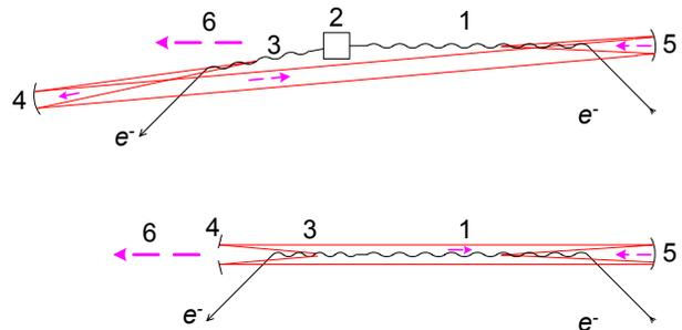
Figure 4: Two schemes of the regenerative amplifier FEL exploiting electron outcoupling technique. Top: with e-beam bending. Bottom: with tapering. 1 – main undulator, 2 – achromatic bend, 3 – last undulator section, 4 and 5 – mirrors, 6 – radiation from the main undulator. Radiation used for feedback is shown by red lines and small violet arrows.
