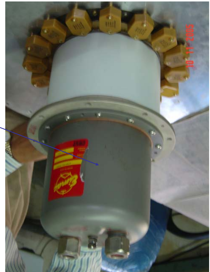
Assembly of Screen By- pass Capacitor with Tetrode
