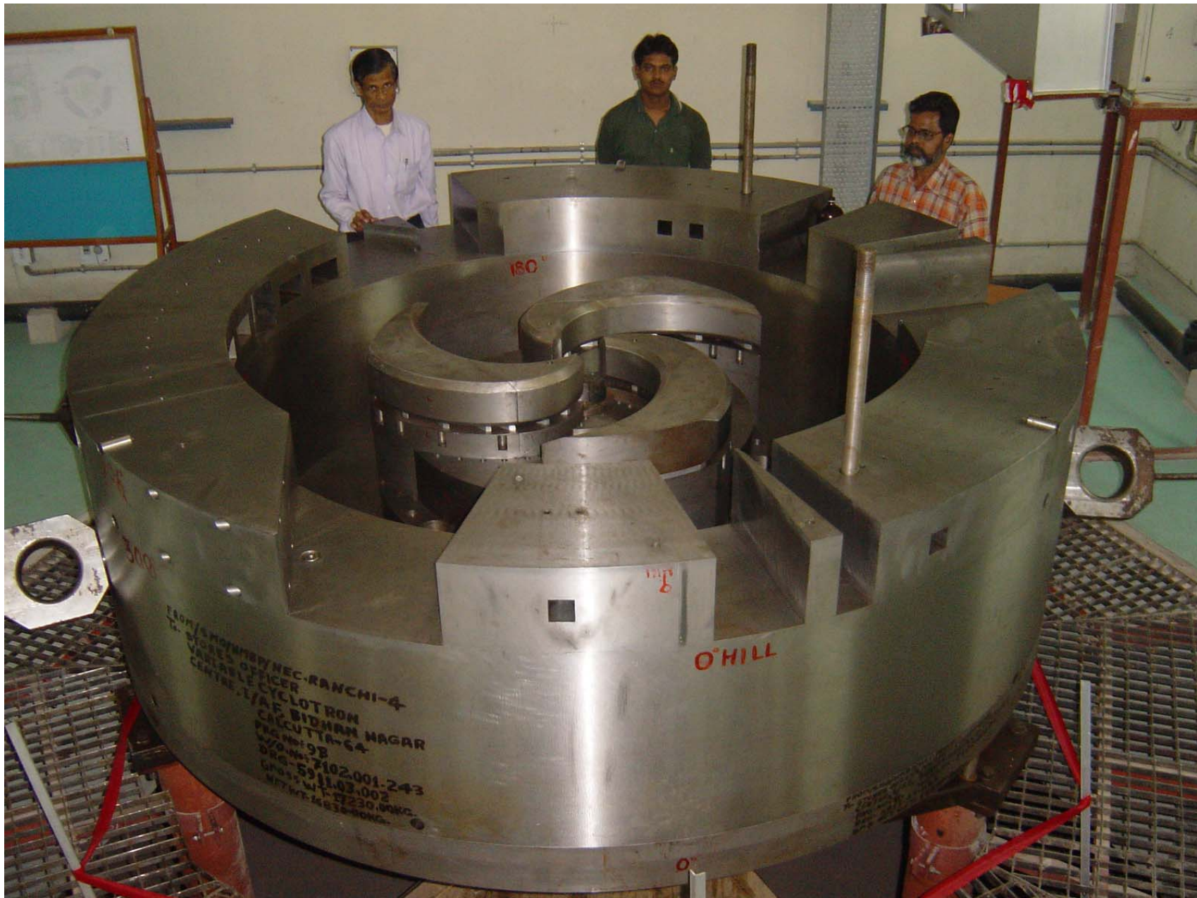
MAGNET ASSEMBLY IS IN PROGRESS
