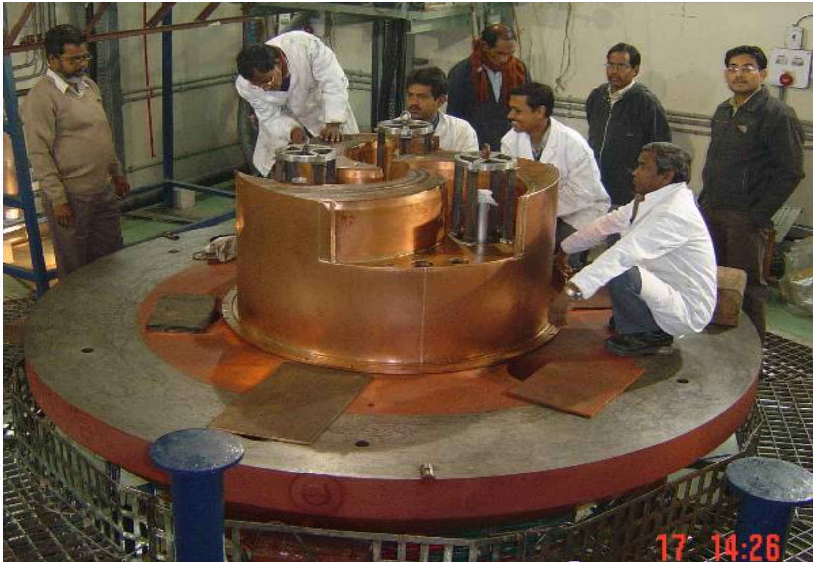
RF liner check assembly
