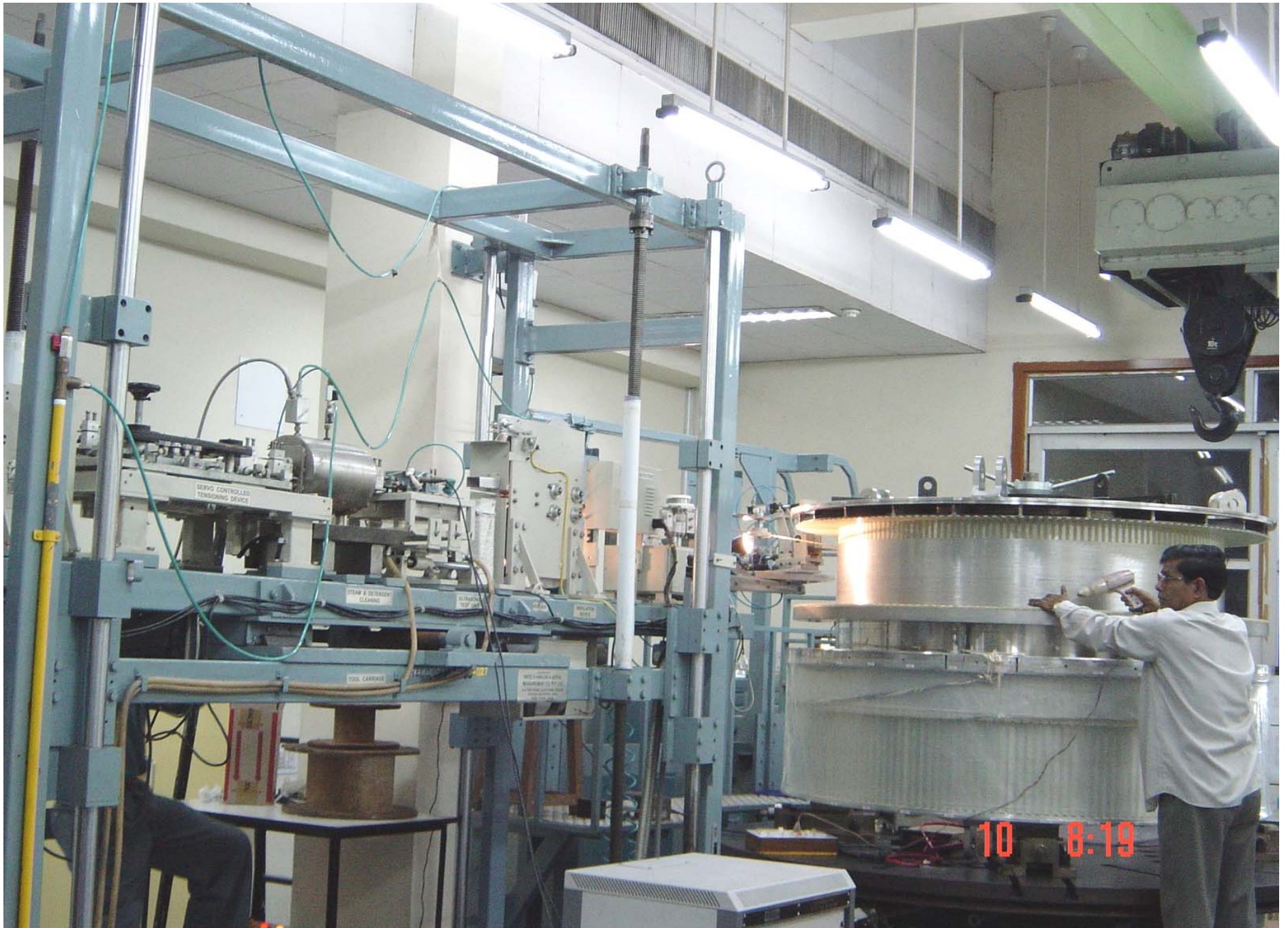
Coil winding in progress
