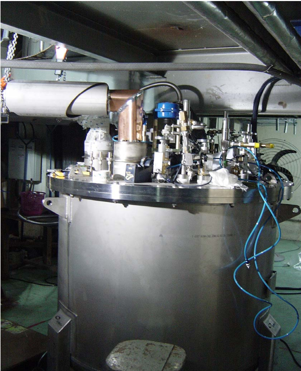
Pump cryostat for LHe delivery to the cryopanel
