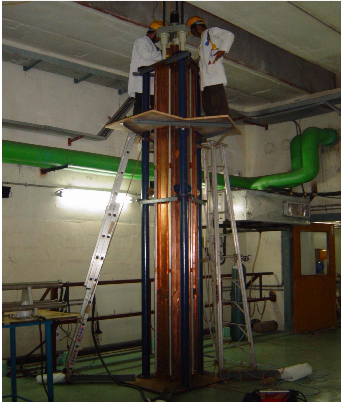
One of the six RF resonators being assembled at VECC
