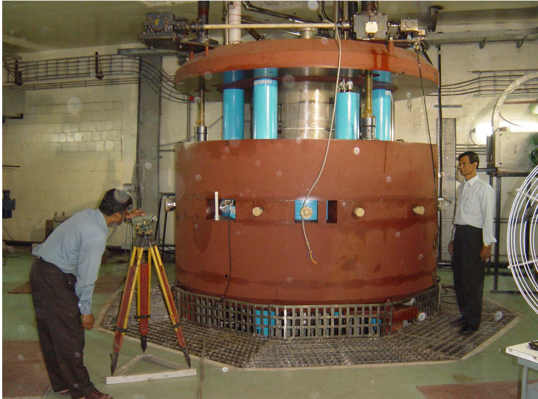
Magnet assembly with pole cap lifted position - maximum lifting height of upper pole cap is 1143mm.
