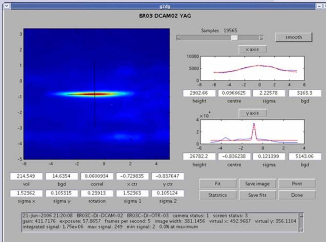
Extracted beam at 3 GeV
