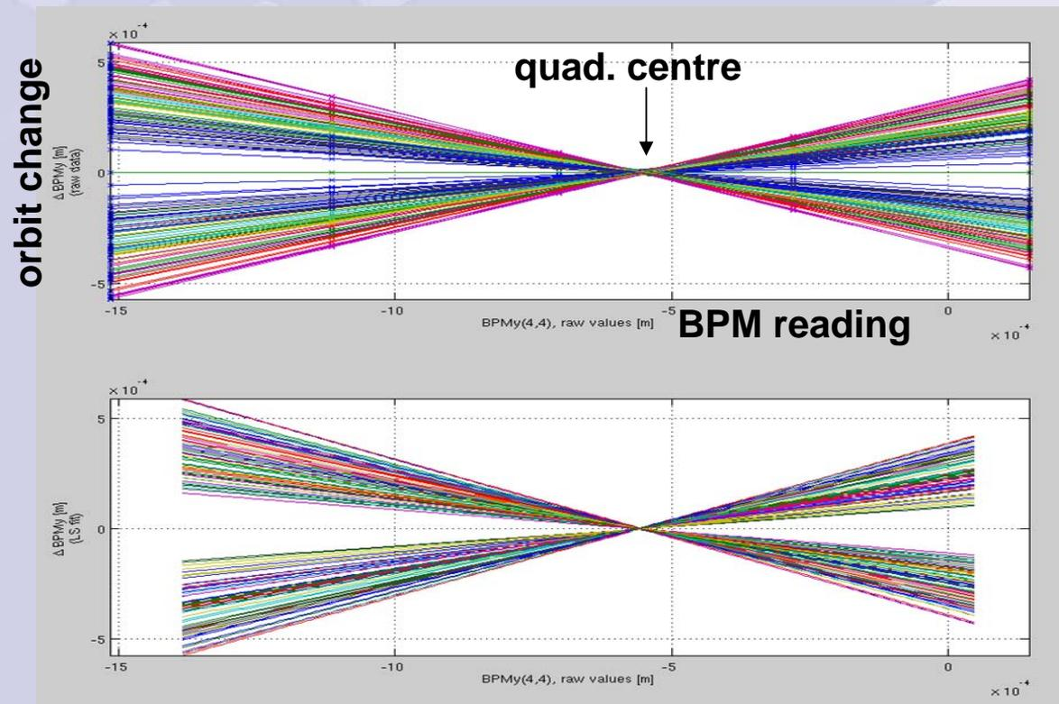
corrector is varied to find the point that the beam passes through the centre of the adjacent quadrupole
