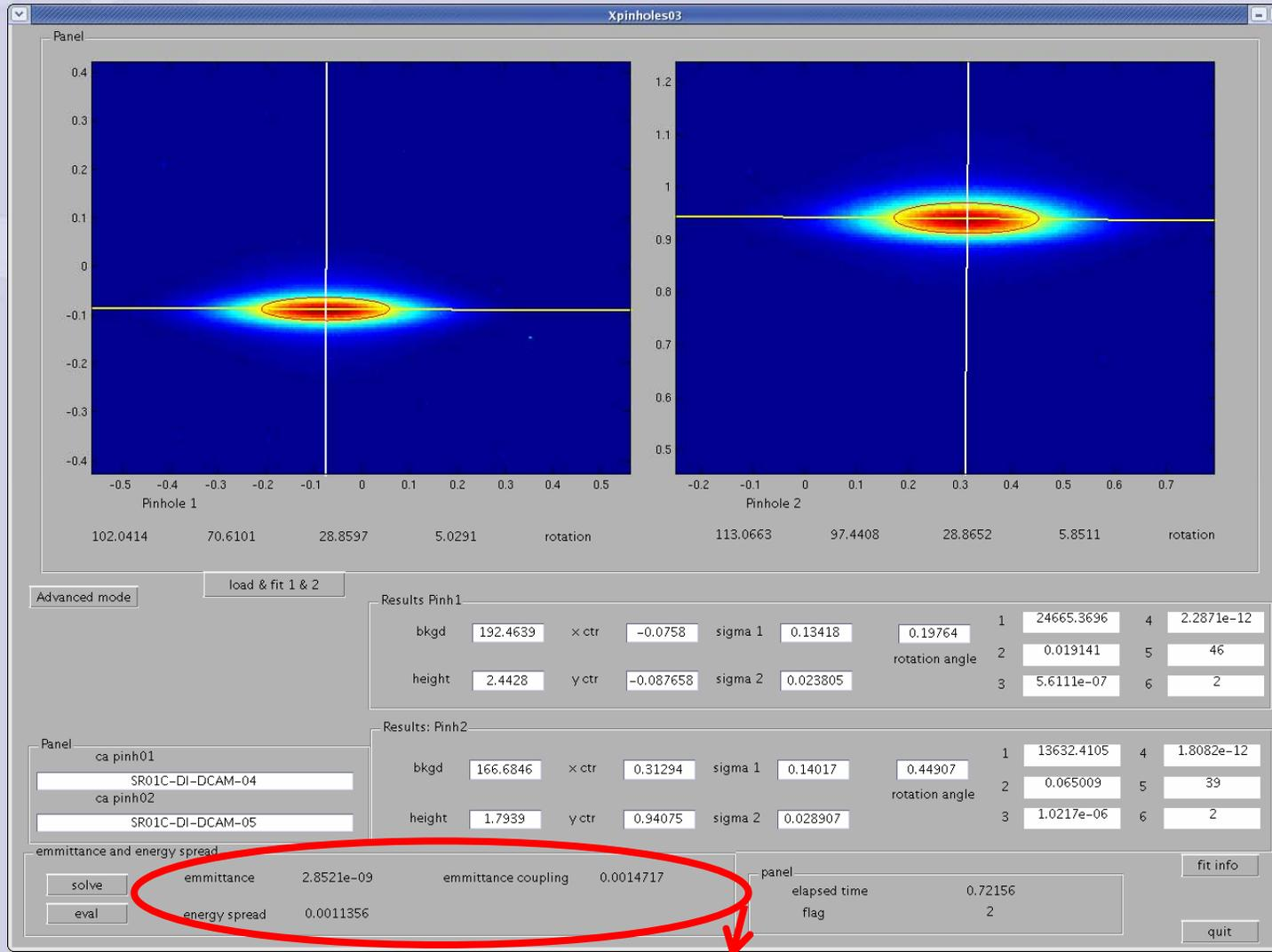
emittance 2.85 nm, energy spread 0.11%, coupling 0.15% (4.2 pm !)
