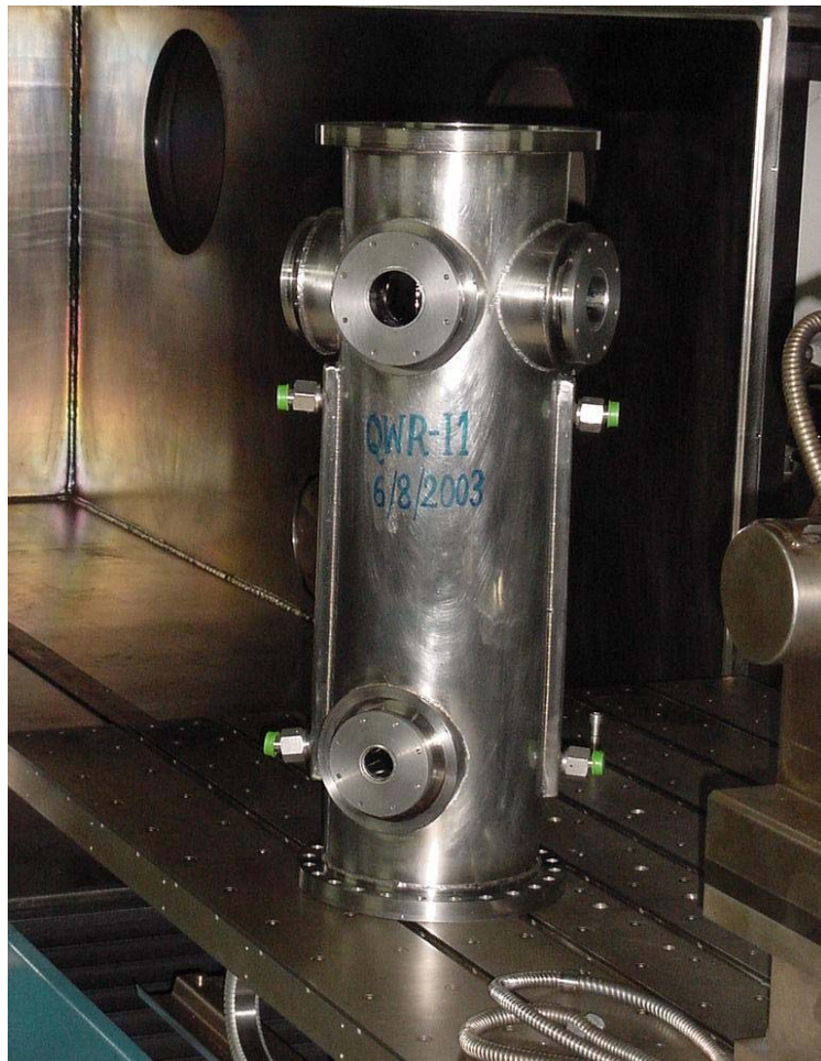
First QWR cavity fabricated at NSC
